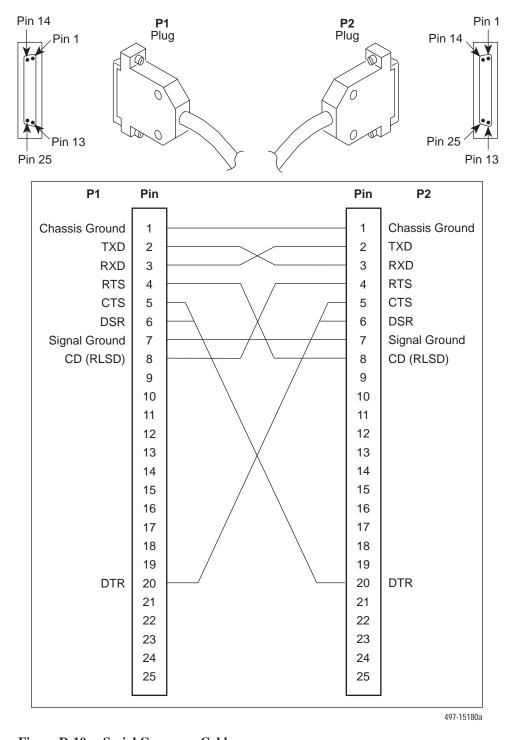
Figure D-10. Serial Crossover Cable
